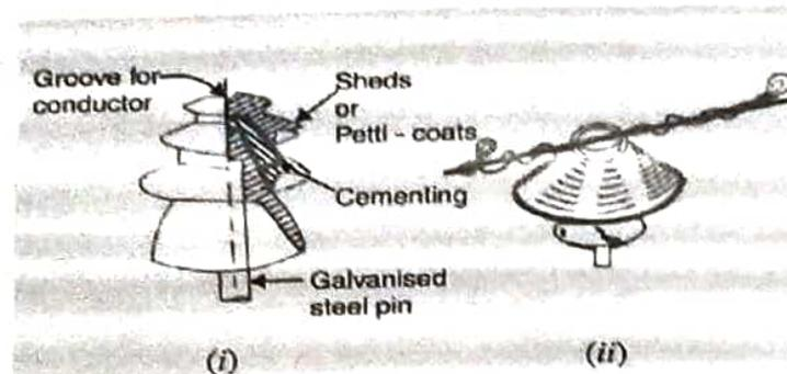
Fig 2.1- Pin Insulator
