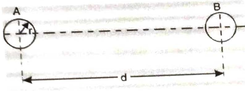
Fig 1.4: Single phase two wire transmission line
