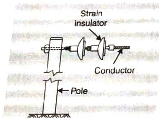
Fig 2.2- Strain Insulator
