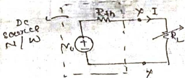
$$I = \frac{V_0}{R_{th} + R_L}$$
