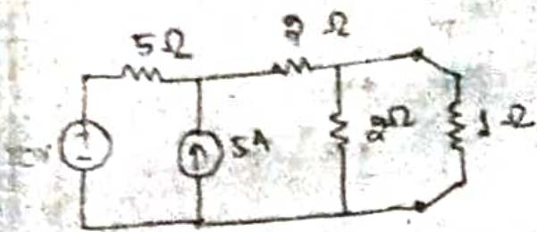
Find power loss in  $1\Omega$  resistor using Norton's theorem.
