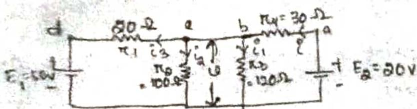
Using Nodal method, find the current through  $R_2$ .
