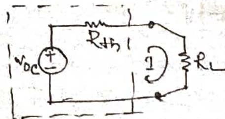
$$\text{The load current } (I) = \frac{V_{oc}}{R_{th} + R_L}$$
