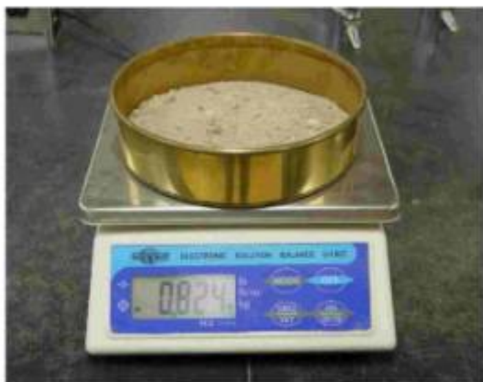
Fig: Illustrates Sieve Analysis test procedure
