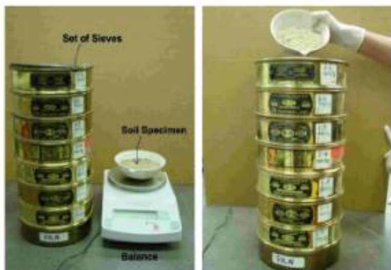
Fig: Illustrates Sieve Analysis test procedure
