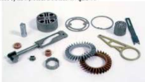
Figure 14: Difficult internal parts made by EDM process
