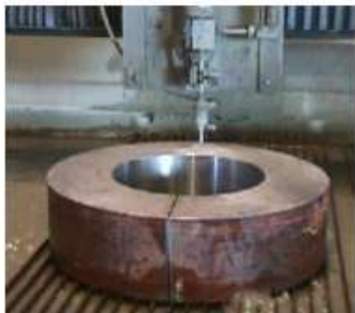
Figure 5: Abrasive water jet cutting
