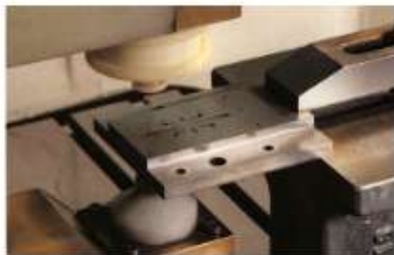
Figure 15: Wire erosion of an extrusion die
