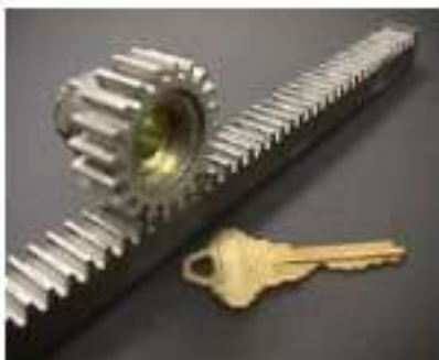
Figure 6: Steel gear and rack cut with an abrasive water jet
