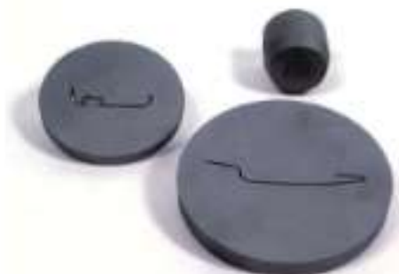
Figure 16: Spark-eroded extrusion dies
